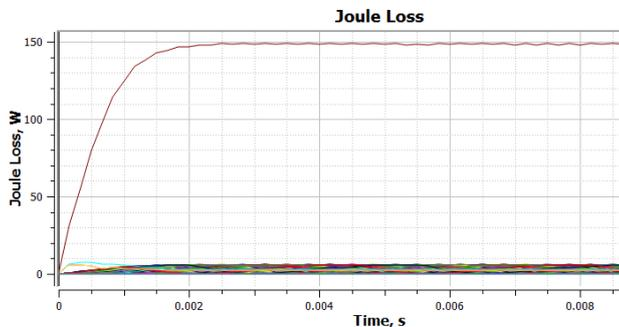
Fig. 2. Joule losses - 500 rpm
