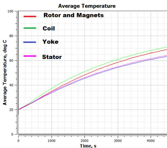
Fig. 5. Thermal study - 360 rpm.
