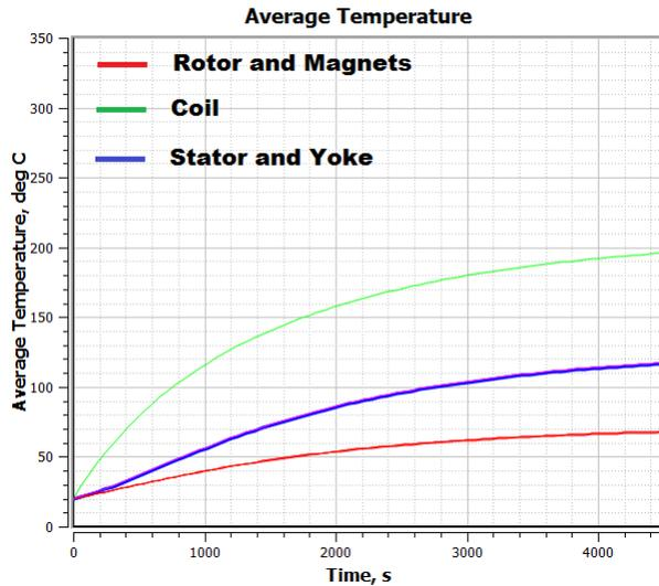
Fig. 7. Thermal analysis - 500 rpm with air dissipation.
