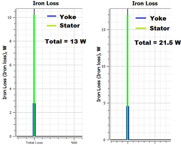
Fig. 6. Iron loss - 250 rpm and 360 rpm.
