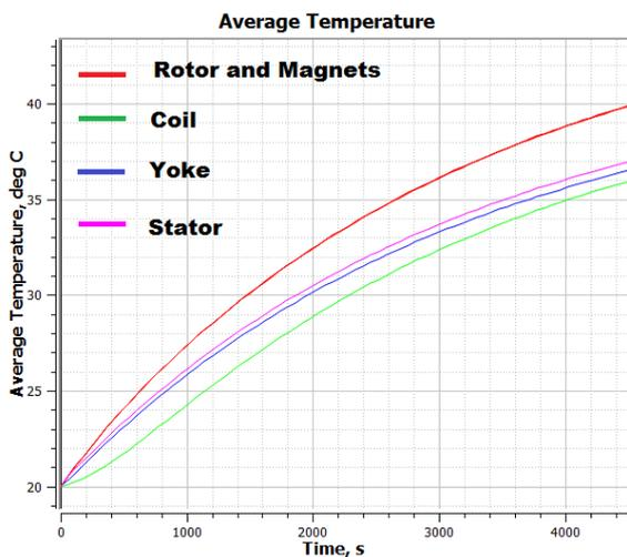
Fig. 4. Thermal study - 250 rpm.
